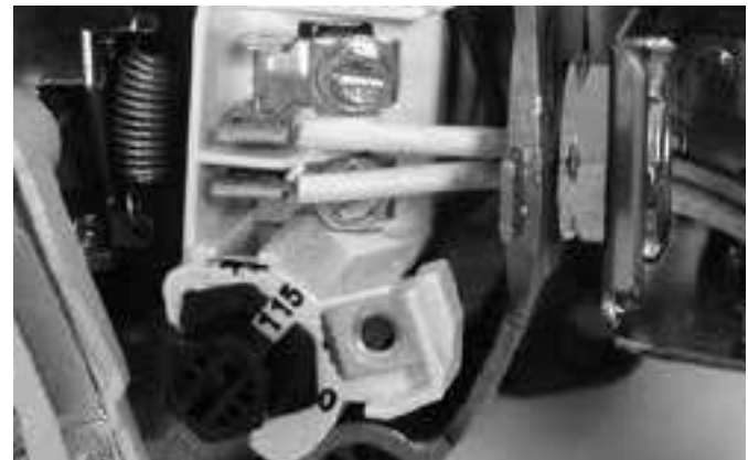
Figure 9 - Voltage set to 115 V, Dial Type
